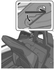
4. Remove the L-shaped hexagonal wrench (Large) once from the bolt, then insert the long end of the wrench into the bolt.
