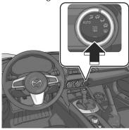
The rear window defogger operates and the switch indicator light turns on.
