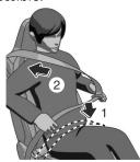
6. The belt should not touch the neck, jaw, or face and it should pass over the shoulder.
