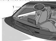
1. Forward Sensing Camera (FSC)
