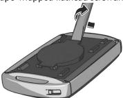
6. Remove the battery using the tape-wrapped flathead screwdriver.
