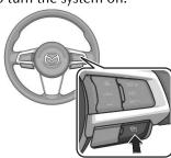
When the system is on, the MRCC standby indication (white) is displayed on the screen.
