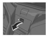
Insert the auxiliary key and turn it clockwise to lock, counterclockwise to unlock.
