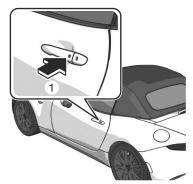
1. Request switch The following locations are locked by pressing the request switch.
