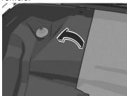
14. Pull out the cap and release the trunk lock. After performing this emergency measure, have the vehicle inspected at an Authorized Mazda Dealer as soon as possible.
