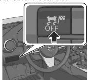
Press the DSC-TRACK switch again to stop the DSC-TRACK operation. For the TCS/DSC/KPC operation condition, refer to How to Use the Dynamic Stability Control (DSC) 5-66.
