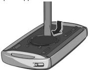
7. Insert a new battery into the key so that the positive pole is facing up.
