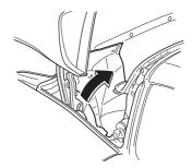
8. Insert your hand beneath the lifted cover and loosen the cap screws until they spin freely.
