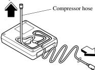
8. Install the air compressor hose which was pulled out of the air compressor to the injection valve of the bottle.
