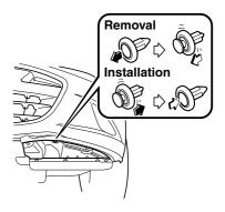
Turn the screw counterclockwise and remove it, and then partially peel back the mudguard.
