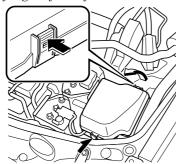
3. Remove the cover while lifting it and sliding it to the rear.
