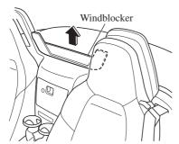
13. Partially peel back the cover on the right side from the middle of the vehicle.
