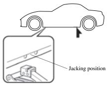
5. Continue raising the jack head gradually by rotating the screw with your hand until the jack head is inserted into the jack-up position.
