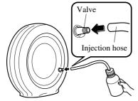
11. Hold the bottom of the bottle upright, squeeze the bottle with your hands, and inject the entire amount of tire sealant into the tire.
