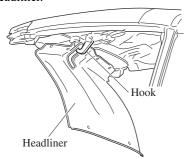
11. Turn the hexagonal wrench (Small) and gear (tool kit) counterclockwise and engage the hook with the vehicle body side.
