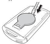
6. Remove the battery using tape-wrapped flathead screwdriver.
