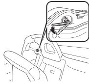
4. Remove the L-shaped hexagonal wrench (Large) once from the bolt, then insert the long end of the wrench into the bolt.
