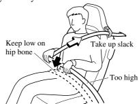
Before fastening the seat belt, make sure that the seat belt passes through the seat belt guide correctly and it is not twisted.
