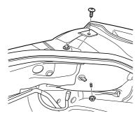
8. To remove the rear combination lamp unit, insert your finger from inside the trunk and into the hole from which the grommet was removed in Step 5, and while holding the lamp lens (round part) of the rear combination lamp with your hand, press the rear combination lamp unit until the hook detaches from the clip.
