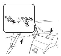
6. Push the stopper rubber through the cover on the right side of the vehicle while slightly lifting the cover up.
