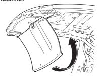
13. Install the headliner to the front roof using the fasteners at two locations.
