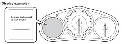
If the warning light turns on/flashes simultaneously or a symbol is indicated in the display, check the information regarding the warning light or symbol.
