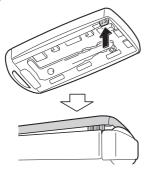
3. Insert a tape-wrapped flathead screwdriver into the gap and slide it in the direction of the arrow.
