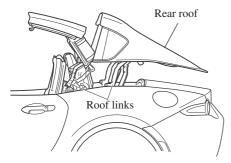
6. After cleaning the drainage outlets, continuously press the retractable hardtop switch in the close direction to close the rear roof.
