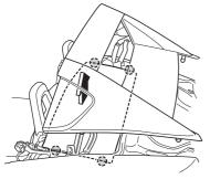
2. Switch your hand on the rear side of the front roof to the front side and pull the front roof forward.
