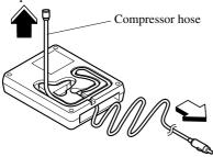
17. Install the air compressor hose to the tire valve.
