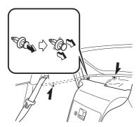
4. Push the stopper rubber through the cover on the right side of the vehicle while slightly lifting the cover up.
