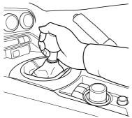
· If shifting to R is difficult, shift back into neutral, release the clutch pedal, and try again.
