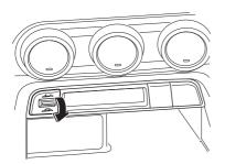
7. Pour about 200 ml (200 cc) of water at once into each of the left and right drainage outlets to wash away small particles of foreign matter inside the drainage path.
