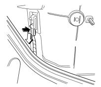
4. Pull the center of each plastic retainer and remove the retainers, and then partially peel back the trunk side trim.
