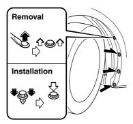
4. Remove the unit by pressing the tab on the unit with your finger and pulling the unit forward.
