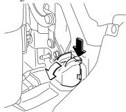
3. Remove drain filter B out of the opening after removing drain filter A.
