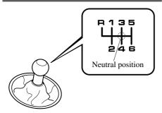
The shift pattern of the transmission is conventional, as shown.
