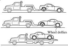
When towing with the rear wheels on the ground, release the parking brake.
