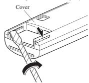
3. Insert the tape-wrapped flathead screwdriver into the gap and slide it in the direction of the arrow.
