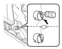
7. Pull out the cap and release the trunk lock.
