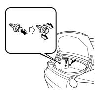
Partially peel back the cover inside the trunk, then pull the emergency release lever.
