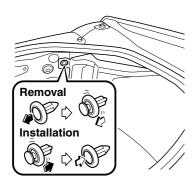
5. To provide a hole for inserting a finger to remove the rear combination lamp unit later in the procedure, pinch the top and bottom of the grommet shown in the figure and press it out of the hole in the direction of the rear combination lamp unit.
