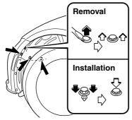
4. Disconnect the connector from the unit by pressing the tab on the connector with your finger and pulling the connector rearward.
