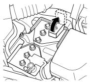
4. Turn off the booster vehicle's engine and connect the jumper cables in the following order.
