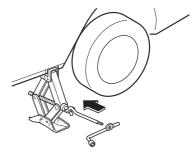
7. Turn the jack handle clockwise and raise the vehicle high enough so that the tire is raised off the ground and can be removed. Before removing the lug nuts, make sure your Mazda is firmly in position and that it cannot slip or move.
