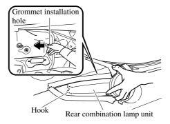
After the hook is detached, pull out the rear combination lamp unit in the direction of the arrow and remove it.
