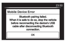
Make sure that the Android<sup>TM</sup> Smartphone in question is compatible with Android Auto<sup>TM</sup>. Before trying to reconnect your Android<sup>TM</sup> Smartphone to the connector cord, do the Bluetooth<sup>®</sup> device pairing again.
