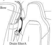
2. Remove the drain filter A while pressing the tab.
