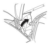
6. Insert your hand beneath the lifted cover and loosen the cap screws until they spin freely.
