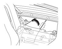
14. Pull out the cap and release the trunk lock.
