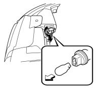
12. Install the new bulb in the reverse order of the removal procedure.
