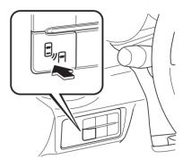
When the Blind Spot Monitoring (BSM) switch is pressed, the Blind Spot Monitoring (BSM) and Rear Cross Traffic Alert (RCTA) systems are turned off and the Blind Spot Monitoring (BSM) OFF indicator light in the instrument cluster turns on.
