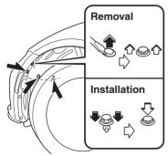
4. Turn the socket and bulb assembly counterclockwise and remove it.
