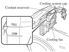
If it is at or near LOW, add enough coolant to the coolant reservoir to provide freezing and corrosion protection and to bring the level to FULL.
