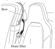
2. Remove the drain filter while pressing the tab.
