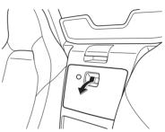
To open, press the latch down to open the seat side box.
