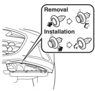
3. Turn the screw counterclockwise and remove it, and then partially peel back the mudguard.
