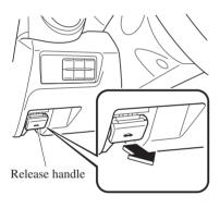
2. Insert your hand into the hood opening, slide the latch lever to the right, and lift up the hood.
