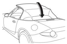
8. With the back end of the convertible top pressed, press the front end until a latch sound is heard.
