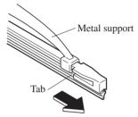
3. Remove the metal stiffeners from each blade rubber and install them in the new blade.
