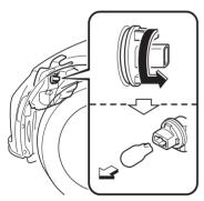
7. Install the new bulb in the reverse order of the removal procedure.
