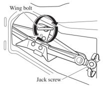
3. Turn the wing bolt completely to secure the jack.
