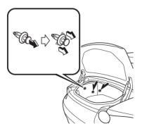
3. Partially peel back the cover inside the trunk, then pull the emergency release lever
