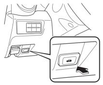
The remote release button function can be disabled by locking the doors using the transmitter, auxiliary key, or a request switch to prevent an intruder in the vehicle from opening the trunk.
