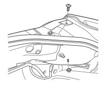
8. To remove the rear combination lamp unit, insert your finger from inside the trunk and into the hole from which the grommet was removed in Step 5, and while holding the lamp lens (round part) of the rear combination lamp with your hand, press the rear combination lamp unit until the hook detaches from the clip.
