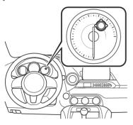
14. Adhere the repaired tire sticker to the wheel of the flat tire.
