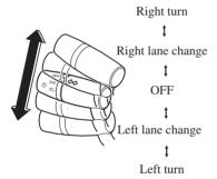
The turn signal indicators in the instrument cluster flash according to the operation of the turn signal lever to show which signal is working.
