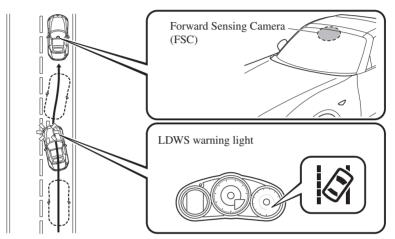
The warning light illuminates when the system has a malfunction. Refer to Warning Lights on page 4-16.
