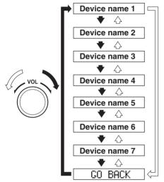
5. Press the audio control dial to select the device you would like to link. The symbol disappears, and "PAIRING" flashes in the audio display.
