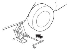
7. Turn the jack handle clockwise and raise the vehicle high enough so that the tire is raised off the ground and can be removed. Before removing the lug nuts, make sure your Mazda is firmly in position and that it cannot slip or move.
