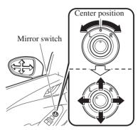
After adjusting the mirror, lock the control by rotating the switch in the center position.
