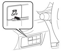
Press the switch again to turn the TCS/DSC back on. The DSC OFF indicator light will turn off.
