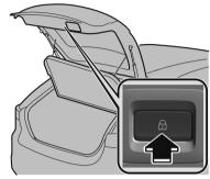
When locking using the door-lock switch, press the door-lock switch with all of the following conditions met and then close the liftgate.
