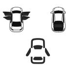
The light turns on if any door/liftgate is not closed securely.
