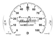
To reset the displayed average energy efficiency data, press the INFO switch for 1.5 seconds or longer. After resetting the data, - - - kWh/100 km (- - - mile/kWh) is displayed before the average energy efficiency is recalculated and displayed.
