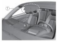
1. Forward Sensing Camera (FSC)
