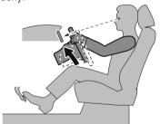
3. Raise the lever to securely lock the steering wheel.
