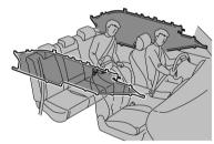
Both curtain air bags will deploy after the roll-over accident is detected.
