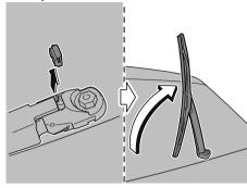
3. Firmly rotate the wiper blade to the right until it unlocks, then remove the blade.
