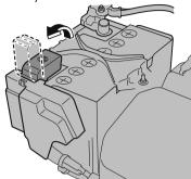
4. Turn off the booster vehicle's engine and connect the jumper cables in the following order.
