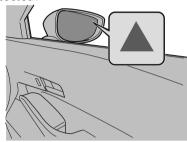
When the power switch is switched ON, the warning indicator light turns on momentarily and then turns off after a few seconds.
