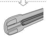
Pull the end of the blade rubber from the blade holder groove in the direction of the arrow and remove the blade rubber from the blade holder.
