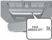
If the front passenger weight sensors are normal, the indicator light illuminates when the power switch is switched ON. The light turns off after a few seconds. Then, the indicator light illuminates or is off under the following conditions:
