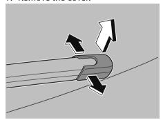
2. Remove the stopper and raise the wiper arm.
