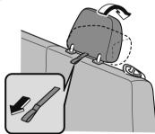
To return the head restraint to its upright position, lift it upward. After lifting up the head restraint to its original position, make sure that it is secured by lightly moving it forward and back.
