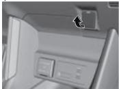
2. Pass the connection plug cord through the cutout of the console and insert the plug into the accessory socket.
