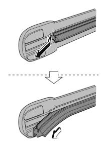
Insert the end of the new blade rubber into the groove of the blade holder until it contacts the end of the blade holder.
