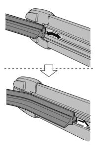
7. After pulling the blade rubber in the direction of the arrow and sliding the blade rubber to a position to check the blade holder groove, slide the blade rubber end in the opposite direction.
