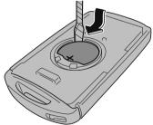
Insert a new battery into the transmitter so that the positive pole is facing up.
