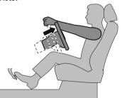
Adjust the steering wheel height so that the gauges can be viewed easily.
