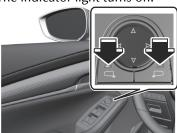
3. Press the adjustment switch to adjust the angle of the outside mirror.
