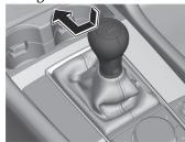
3. Release the clutch pedal. The Gear Shift Indicator (GSI) is displayed in the instrument cluster. Refer to Gear Shift Indicator (GSI) on page 5-53.
