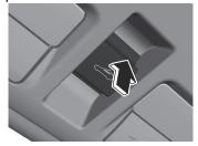
3. Press the tilt/slide switch forward.
