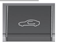
The mode is switched between recirculate mode and fresh air mode each time the switch is pressed. The display indicates whether recirculate mode (<a>) or fresh air mode ( $\Leftrightarrow$ ) is selected.
