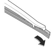
5. Remove the metal stiffeners from the blade rubber and install them in the new blade rubber.
