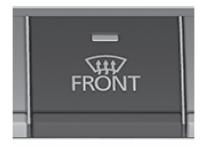
Switches the windshield defroster on (indicator light turned on) and off (indicator light turned off).
