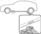
6. Continue raising the jack head gradually by rotating the screw with your hand until the jack head is inserted into the jack-up position.
