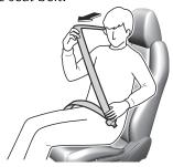
If the belt is locked and cannot be pulled out, retract the belt once, and then try pulling it out slowly. If this fails, pull the seat belt strongly one time and loosen it, then pull it out again slowly.
