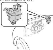
If it is at or near the LOW position, add enough coolant to the coolant reservoir to provide freezing and corrosion protection and to bring the level to FULL.
