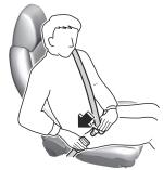
5. The belt should fit the pelvis as low as possible.
