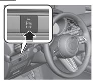
The parking sensors turn off and the parking sensor OFF switch indicator light turns on.
