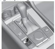
When the parking brake is released, the EPB indicator light PARK in the instrument cluster and the EPB switch indicator light turn off.
