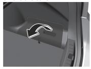
3. Turn the wing bolt and jack screw counterclockwise.
