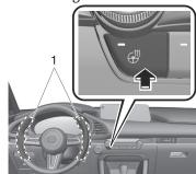
1. Heating area The indicator light in the heated steering wheel switch turns on.
