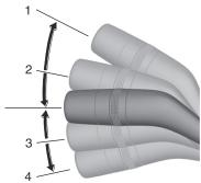
Each turn signal light flashes and the turn signal light  $\Leftrightarrow$  in the instrument cluster flashes. The lever returns to its original position in conjunction with the steering wheel operation. If it does not return, return it by hand.
