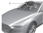
1. Forward Sensing Camera (FSC)
