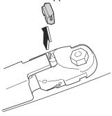
3. Raise the wiper arm and rotate the wiper blade to the right until it unlocks, then remove the blade.
