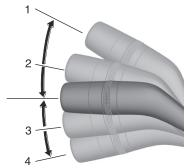
While the lever is in the 2 or 3 position, each turn signal light flashes and the turn signal light  $\diamondsuit$  in the instrument cluster flashes. If you move the lever to the 2 or 3 position and release it immediately, the three-flash turn signal operates and the turn signal light flashes 3 times.
