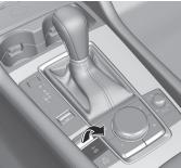
When the shift-linked release is enabled, a sound is activated 2 times, the EPB switch indicator light switches to fast flashing, and then flashes for a certain period of time.
