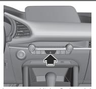
All the turn signal lights flash and the turn signal light in the instrument cluster flashes.
