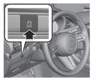
The TCS/DSC operation is canceled and the DSC OFF indicator light in the instrument cluster turns on. Press the DSC OFF switch again to enable the TCS/DSC operation.
