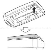
3. Insert a tape-wrapped flathead screwdriver into the gap and slide it.
