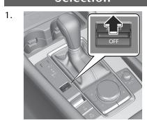
When the sport mode is selected, the select mode indicator light **SPORT** turns on in the instrument cluster.
