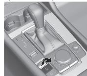
The parking brake is applied and the EPB indicator light PARK in the instrument cluster and the EPB switch indicator light turn on.
