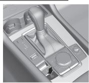
The AUTOHOLD becomes operational and the AUTOHOLD standby indicator light turns on.
