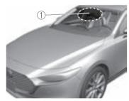
1. Forward Sensing Camera (FSC)
