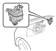
If it is at or near LOW, add enough coolant to the coolant reservoir to provide freezing and corrosion protection and to bring the level to FULL.
