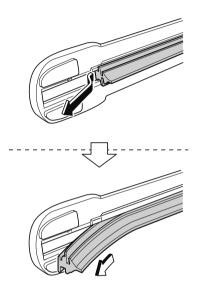
6. Insert the end of the new blade rubber into the groove of the blade holder until it contacts the end of the blade holder.
