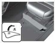
When setting a floor mat, position the floor mat so that its grommets are inserted over the pointed end of the retention posts.
