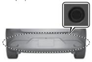
The ultrasonic sensors are mounted in the rear bumper.
