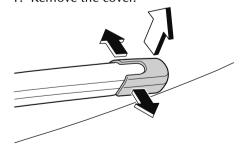
2. Remove the stopper and raise the wiper arm.
