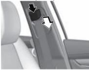
After adjusting, press the front shoulder belt adjuster downward and make sure that it is securely locked.
