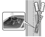
1. Forward sensing camera (FSC)
