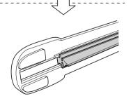
5. Pull the end of the blade rubber from the blade holder groove in the direction of the arrow and remove the blade rubber from the blade holder.
