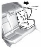
5. Push the child-restraint system firmly into the vehicle seat. Be sure the belt retracts as snugly as possible. A clicking noise from the retractor will be heard during retraction if the system is in the automatic locking mode. If the belt does not lock the seat down tight, repeat this step.
