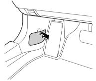
3. Pull the fuse straight out with the fuse puller provided on the fuse block located in the engine compartment.
