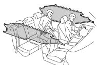
Both curtain air bags will deploy after the roll-over accident is detected.
