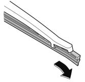
5. Remove the metal stiffeners from the blade rubber and install them in the new blade.
