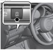
Press the switch again to turn the TCS/DSC back on. The DSC OFF indicator light will turn off.
