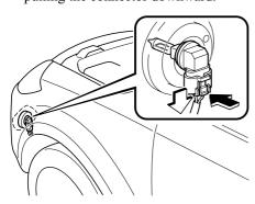
5. Turn the socket and bulb assembly counterclockwise and remove it.
