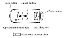
A code number is stamped on the plate attached to the key set; detach this plate and store it in a safe place (not in the vehicle) for use if you need to make a replacement key.
