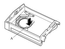
5. Put in the new battery (CR1620 or equivalent) with the positive pole (+) facing down.
