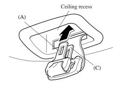
To pull out the seat belt, press the area indicated in the figure upward with your finger and slide the belt forward. Then slowly pull out the seat belt from the ceiling recess.
