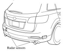
Always keep the bumper surface near the radar sensor area clean so that the BSM system operates normally. Refer to the Exterior Care (page 8-56).
