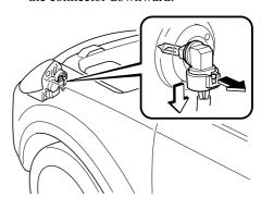
Turn the socket and bulb assembly to remove it. Carefully remove the bulb from its socket in the reflector by gently pulling it straight backward out of the socket.
