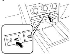
Press the seat warmer switch to illuminate the indicator light while the ignition is switched ON. The mode changes as follow each time the seat warmer switch is pressed.
