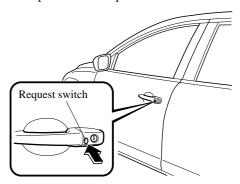
To stop the windows and the moonroof from closing, release the request switch. If the operation is performed from the beginning again, the windows and the moonroof close.
