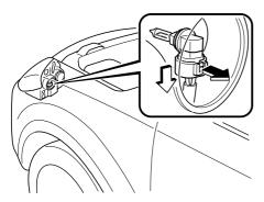
Turn the socket and bulb assembly to remove it. Carefully remove the bulb from its socket in the reflector by gently pulling it straight backward out of the socket.
