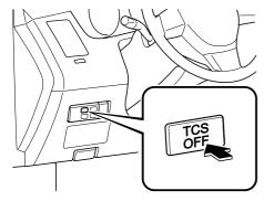
Press the switch again to turn the TCS back on. The TCS OFF indicator light will turn off. If the vehicle speed is more than 15 km/h (9 mph), the TCS OFF indicator light will not illuminate even if the switch is pressed.
