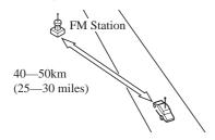
Signals from an FM transmitter are similar to beams of light because they do not bend around corners, but they do reflect. Unlike AM signals, FM signals cannot travel beyond the horizon. Therefore, FM stations cannot be received at the great distances possible with AM reception.
