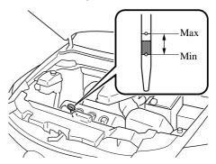
5. Pull it out again and examine the level. The level is normal if it is between MIN and MAX. If it is below MIN, add oil to raise the level within the hatching zone.
