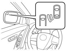
This warning light illuminates for a few seconds when the ignition is switched ON.
