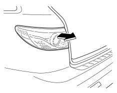
4. Turn the socket and bulb assembly counterclockwise and remove it.
