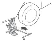
Turn the jack handle clockwise and raise the vehicle high enough so that the spare tire can be installed. Before removing the lug nuts, make sure your Mazda is firmly in position and that it cannot slip or move.
