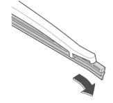
5. Remove the metal stiffeners from the blade rubber and install them in the new blade rubber.
