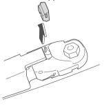
3. Raise the wiper arm and rotate the wiper blade to the right until it unlocks, then remove the blade.
