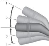
While the lever is in the 2 or 3 position, each turn signal light flashes and the turn signal light in the instrument cluster flashes.
