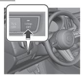
The i-stop function stops and the i-stop OFF switch indicator light turns on.
