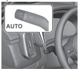
The HBC determines the surrounding conditions and operates automatically. When the HBC operates, the HBC indicator light (green) in the instrument cluster turns on.
