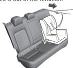
6. Push the child-restraint system firmly into the vehicle seat. Be sure the belt retracts as snugly as possible. A clicking noise from the retractor will be heard during retraction if the system is in the automatic locking mode. If the belt does not lock the seat down tight, repeat this step.
