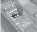
The gear position can be switched manually in manual shift mode. The manual shift mode indication and the gear position are displayed in the instrument cluster.
