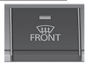
Switches the windshield defroster on (indicator light turned on) and off (indicator light turned off).
