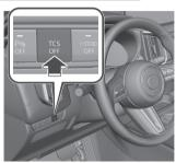
The TCS operation is canceled and the TCS OFF indicator light of in the instrument cluster turn on.
