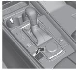
The parking brake is applied and the EPB indicator light PARK in the instrument cluster and the EPB switch indicator light turn on.
