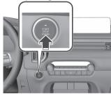
The engine stops and the vehicle power is switched OFF.
