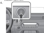
The engine starts and the KEY indicator light (green) <sup>□</sup> in the instrument cluster turns off
