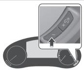
If you press the - switch again while the dashboard illumination is at maximum dimness, a sound is activated to notify you that the dimmer setting is at maximum dimness.
