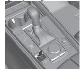
When the parking brake is released, the EPB indicator light has in the instrument cluster and the EPB switch indicator light turn off.
