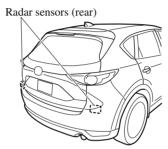
The radar sensors (rear) are installed inside the rear bumper, one each on the left and right sides.
