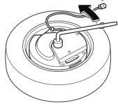
For vehicles not equipped with a sub-woofer, turn the spare tire hold-down bolt counterclockwise and remove the spare tire.
