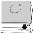
10. Insert the tabs of the lower cover into the slots of the transmitter and install the lower cover.
