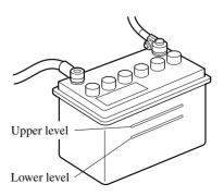
Inspect the electrolyte level at least once a week. If it is low, contact an Authorized Mazda Dealer for the electrolyte level.
