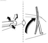
2. Firmly rotate the wiper blade to the right until it unlocks, then remove the blade.
