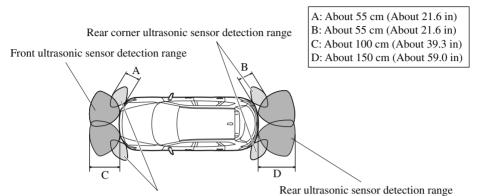
Front corner ultrasonic sensor detection range
