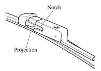
10. Slide the blade component and install it to the wiper arm.
