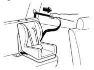
6. Push the child-restraint system firmly into the vehicle seat. Be sure the belt retracts as snugly as possible. A clicking noise from the retractor will be heard during retraction if the system is in the automatic locking mode. If the belt does not lock the seat down tight, repeat this step.
