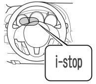
• The i-stop indicator light (green) turns off when the engine is restarted.
