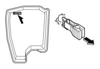
4. Inspect the fuse and replace it if it is blown.
