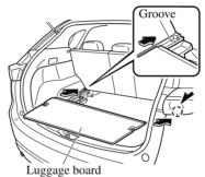
2. Insert the left and right hollows or holes of the rear luggage board into the pins.
