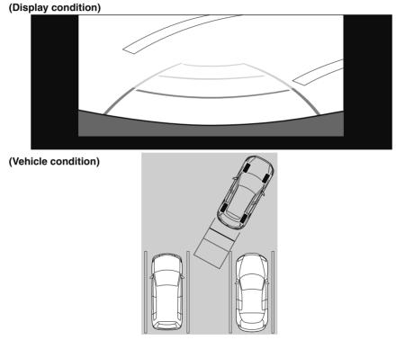
4. Continue to adjust the steering wheel until the vehicle width guide lines are parallel to the left and right sides of the parking space.
