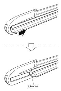
4. Pull the end of the blade rubber from the blade holder groove in the direction of the arrow and remove the blade rubber from the blade holder.
