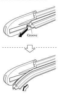
Insert the end of the new blade rubber into the groove of the blade holder until it contacts the end of the blade holder.
