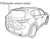
The ultrasonic sensors (rear) are mounted in the rear bumper.
