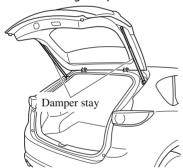
➤ Do not modify or replace the liftgate damper stay. Consult an Authorized Mazda Dealer if a liftgate damper stay is deformed or damaged for reasons such as a collision or if there is some other problem.
