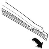
4. Remove the metal stiffeners from the blade rubber and install them in the new blade.
