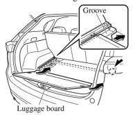
3. Insert the left and right hollows or holes of the rear luggage board into the pins.
