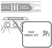
If the front passenger occupant classification sensor is normal, the indicator light turns on when the ignition is switched ON. The light turns off after a few seconds. Then, the indicator light turns on or is off under the following conditions:
