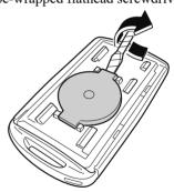
6. Remove the battery using tape-wrapped flathead screwdriver.
