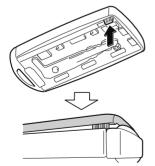
3. Insert a tape-wrapped flathead screwdriver into the gap and slide it in the direction of the arrow.
