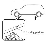
Continue raising the jack head gradually by rotating the screw with your hand until the jack head is inserted into the jack-up position.
