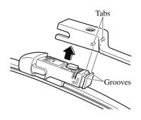
9. Align the blade component projection with the wiper arm notch.
