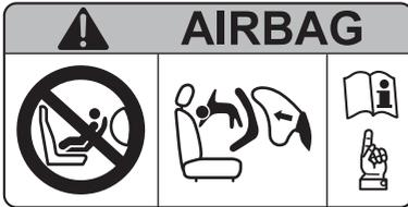
**Do not install a front-facing child-restraint system on the front passenger seat unless it is unavoidable:**
