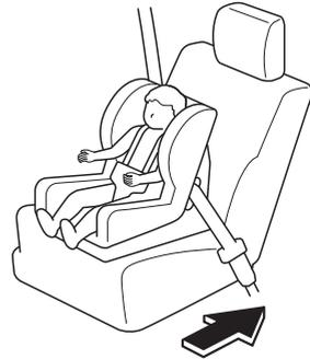
3. Place the child-restraint system on the seat without putting your weight on the seat and fasten the seat belt. See the manufacturer's instructions on the child-restraint system for belt routing instructions.
