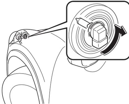
6. Install the new bulb in the reverse order of the removal procedure.
