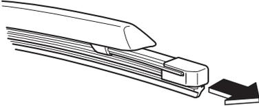
4. Remove the metal stiffeners from each blade rubber and install them in the new blade.
