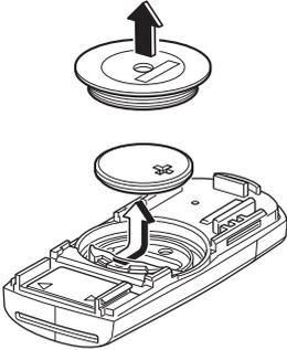
5. Insert a new battery with the positive pole facing up, and then cover the battery with the battery cap.
