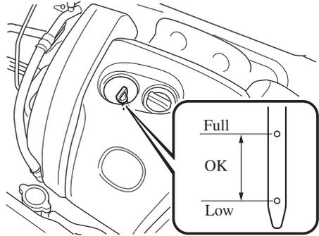
5. Pull it out again and examine the level. The level is normal if it is between Low and Full. If it is near or below Low, add enough oil to bring the level to Full.
