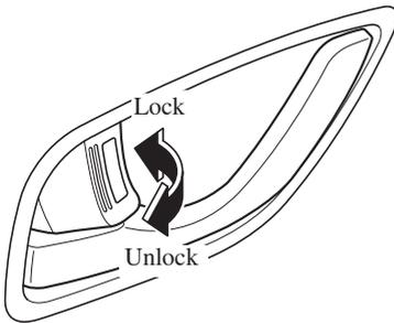
To lock the front passenger door with the door-lock knob from the outside, press the door-lock knob to the lock position and close the door (holding the door handle pulled is not required).
