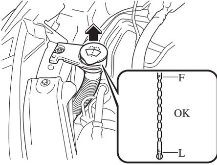
The top of the float should be between F and L.
