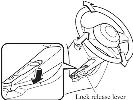
2. Tilt the steering wheel and/or adjust the steering column length to the desired positions, and then push the lever up to lock the column.
