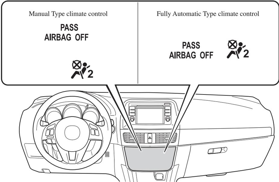
If the front passenger weight sensors are normal, the indicator light illuminates when the ignition is switched ON. The light turns off after a few seconds.
