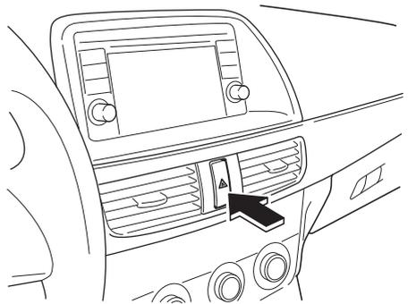
Depress the hazard warning flasher and all the turn signals will flash. The hazard warning indicator lights in the instrument cluster flash simultaneously.
