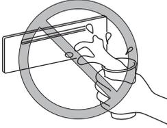
Do not insert any objects, other than CDs, into the slot.
