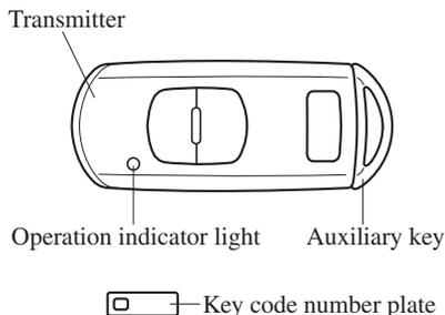
Pull out the auxiliary key from the key (transmitter).
