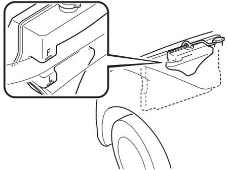
If it is at or near L, add enough coolant to the coolant reservoir to provide freezing and corrosion protection and to bring the level to F.
