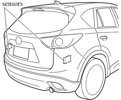
Always keep the bumper surface near the radar sensor area clean so that the BSM system operates normally. Refer to Exterior Care on page 6-56.
