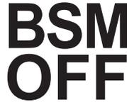
This indicator light illuminates for a few seconds when the ignition is switched ON.
