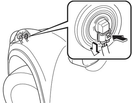
5. Turn the socket and bulb assembly to remove it. Carefully remove the bulb from its socket in the reflector by gently pulling it straight backward out of the socket.
