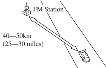
Signals from an FM transmitter are similar to beams of light because they do not bend around corners, but they do reflect. Unlike AM signals, FM signals cannot travel beyond the horizon. Therefore, FM stations cannot be received at the great distances possible with AM reception.
