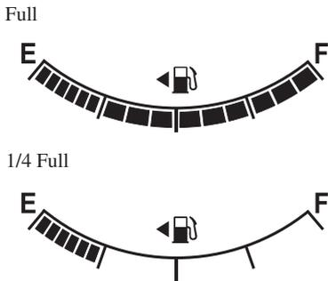
If the low fuel warning light illuminates or the fuel level is very low, refuel as soon as possible.
