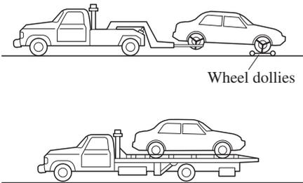
A towed 2WD vehicle should have its drive wheels (front wheels) off the ground. If excessive damage or other conditions prevent this, use wheel dollies.
