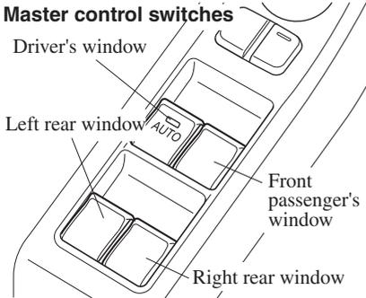
To open the window to the desired position, hold down the switch.
