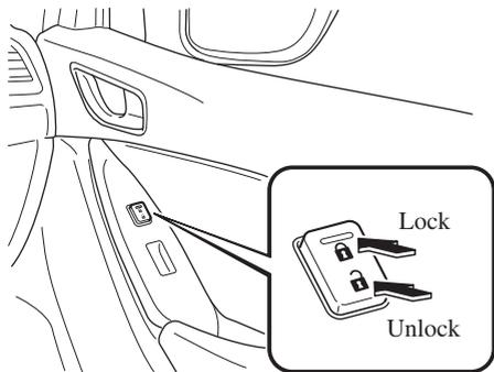
To lock all the doors/liftgate from an open front door, press the lock side of the door lock switch and then close the door.
