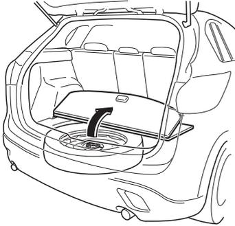
2. Secure the trunk board by attaching the hook to the head restraint.
