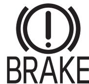
If the brake warning light remains illuminated even though the parking brake is released, the brake fluid may be low or there could be a problem with the brake system. Park the vehicle in a safe place immediately and contact an Authorized Mazda Dealer.
