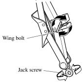
3. Turn the wing bolt completely to secure the jack.
