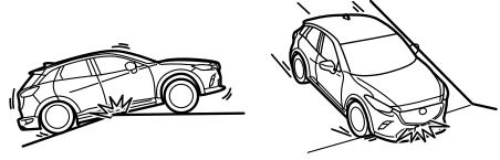
This vehicle is equipped with low profile tires allowing class-leading performance and handling. As a result, the sidewall of the tires are very thin and the tires and wheels can be damaged if driven through potholes or on rough/uneven roads at excessive speeds. Use care and reduce speed when traveling on rough/uneven roads or through potholes.
