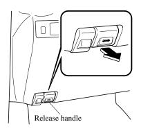
2. Insert your hand into the hood opening, slide the latch lever to the right, and lift up the hood.
