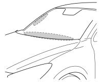
The windshield wiper de-icer operates in conjunction with the rear window defogger.
