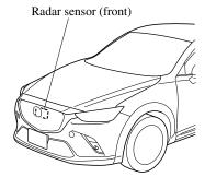
If the Smart Brake Support/Smart City Brake Support (SBS/SCBS) Warning Light (amber) is illuminated, the area around the radar sensor may be dirty. Refer to "Warning Guidance" in the center display (With Mazda Connect).
