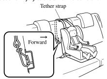
Always attach the tether strap to the correct tether anchor position:
