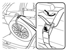
14. Pull the belt end to secure the flat tire.
