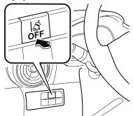
Drive the vehicle in the center of the driving lane while the LDWS OFF indicator light is turned off. The system becomes operational when all of the following conditions are met.
