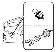
5. Install the new bulb in the reverse order of the removal procedure.
