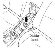
Insert the divider into the armrest from the top with the flap side of the divider facing the underside of the armrest, and press it in until a click sound is heard.
