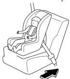
Remove the head restraint. However, when installing a backless booster seat, always install the vehicle head restraint to the seat where the backless booster seat is installed.
