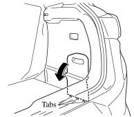
6. Turn the wing bolt and jack screw counterclockwise.
