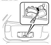
4. Using a flathead screwdriver, turn the lever to the right to unlock the liftgate.
