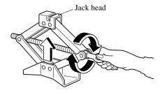
Place the jack under the jack-up position closest to the tire being changed with the jack head squarely under the jack-up point.
