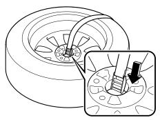
13. Thread the belt through the buckle while pressing the tire to the seatback.
