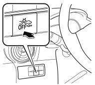
Press the switch again to turn the system back on. The Smart City Brake Support (SCBS) OFF indicator light will turn off.
