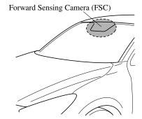
The Forward Sensing Camera (FSC) determines the conditions ahead of the vehicle while traveling at night and detects traffic lanes. The distance in which the Forward Sensing Camera (FSC) can detect objects varies depending on the surrounding conditions.
