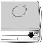
Insert the tabs of the lower cover into the slots of the transmitter and install the lower cover.
