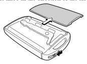
2. Press in the tab to unlock the upper cover.
