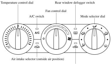
Air intake selector (recirculated air position)
