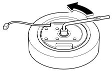
For vehicles not equipped with a sub-woofer, turn the spare tire
