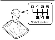
The shift pattern of the transaxle is conventional, as shown.
