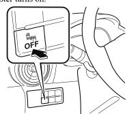
If the switch is pressed again, the BSM and Rear Cross Traffic Alert (RCTA)
