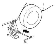
8. Turn the jack handle clockwise and raise the vehicle high enough so that the spare tire can be installed. Before removing the lug nuts, make sure your Mazda is firmly in position and that it cannot slip or move.
