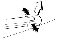
2. Remove the stopper and raise the wiper arm.
