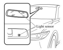
• The auto-dimming function is canceled when the ignition is switched ON and the selector lever is in the R position.
