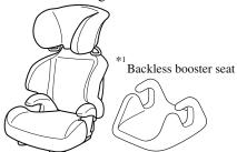
\*1 When using a backless booster seat, always install the vehicle head restraint to the seat where the backless booster seat is installed.
