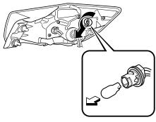
6. Install the new bulb in the reverse order of the removal procedure.
