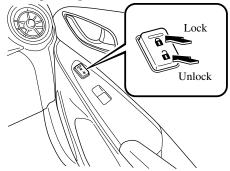
To lock all the doors and the liftgate from an open front door, press the lock side of the door lock switch and then close the door.
