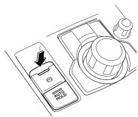
If the EPB switch is pressed without depressing the brake pedal, the indicator light in the instrument cluster notifies the driver that the brake is not depressed.
