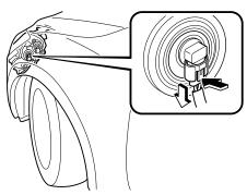
4. Turn the socket and bulb assembly to remove it. Carefully remove the bulb from its socket in the reflector by
