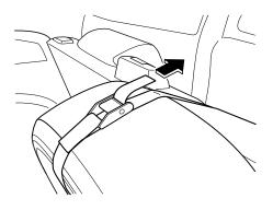
15. Insert the luggage compartment cover from the top of the luggage compartment opening with the cloth side of the cover facing outward, and slide it between the flat tire and the inside perimeter of the luggage compartment opening.
