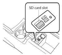
The location of the SD card slot differs depending on the vehicle model.
