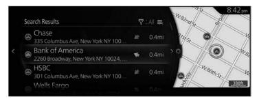
6. Tilt the commander knob to the right and display the option panel to reorder the list from "Sort By" and to limit the area from "Search Area".
