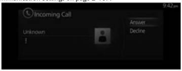
When the conversation begins, press the 30 on the audio remote control switch on the steering wheel control switch, or select "Answer" on the screen.
