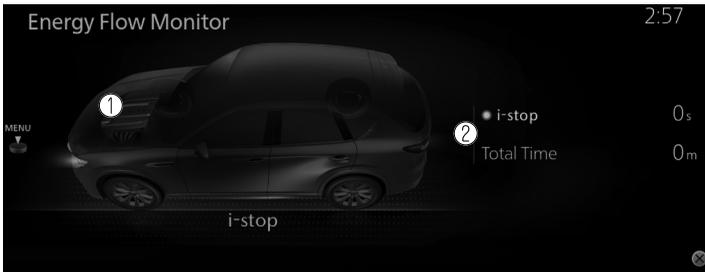
1. Displays the operation status of the i-stop function in the engine area. The engine area is illuminated while the engine idling stop is not operating, and it is not illuminated while the engine idling stop is operating.
